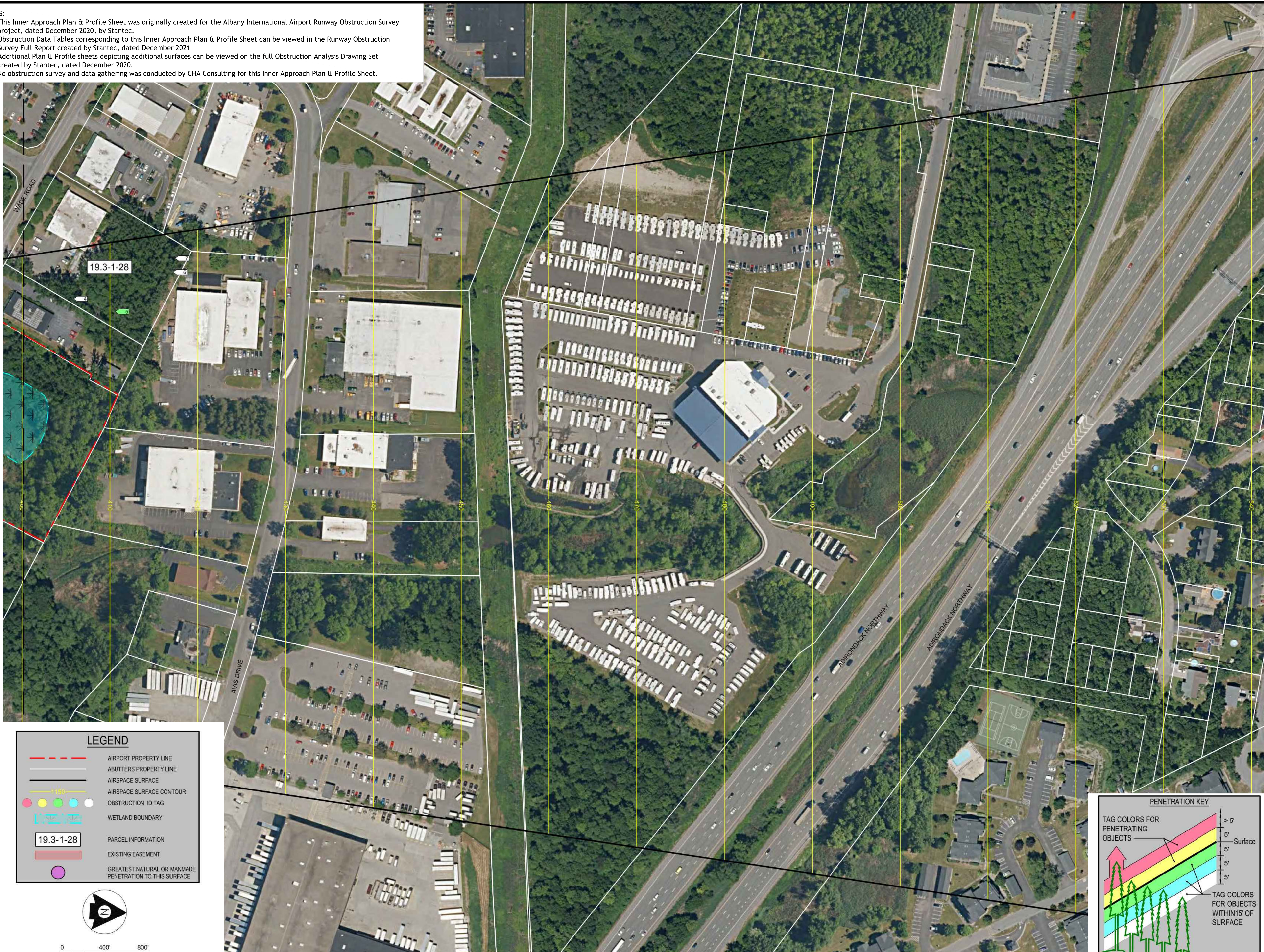
RUNWAY 28 20:1 OBSTACLE CLEARANCE SURFACE (OCS) (NO. 4) & TERPS 20:1 OBSTACLE IDENTIFICATION SURFACE (OIS) ANALYSIS SHEET 2 OF 2
